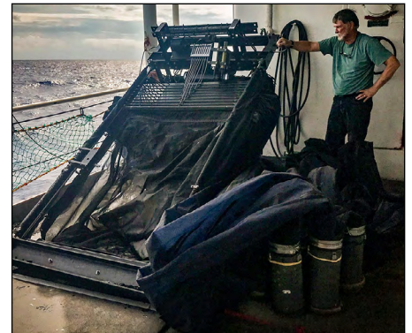
Peter Wiebe stands next to a MOCNESS, which stands for a Multiple Opening/Closing Net and Environmental Sensing System. The MOCNESS net carries anywhere from six to twenty nets, plus electronic sensors for measuring temperature, depth, and salinity. The nets can be opened and closed independently to sample a specific depth of water in the twilight zone, allowing scientists control over where and when they take their samples.
