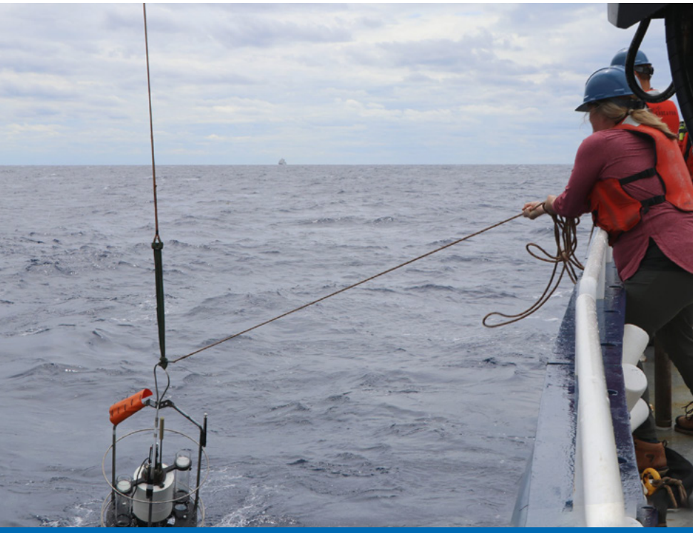
OTZ engineer Kaitlyn Tradd (right) helps to recover TZEX while aboard the R/V Endeavor in August 2022. The instrument features a new rotating marine snow sampler that Tradd designed. © Woods Hole Oceanographic Institution
