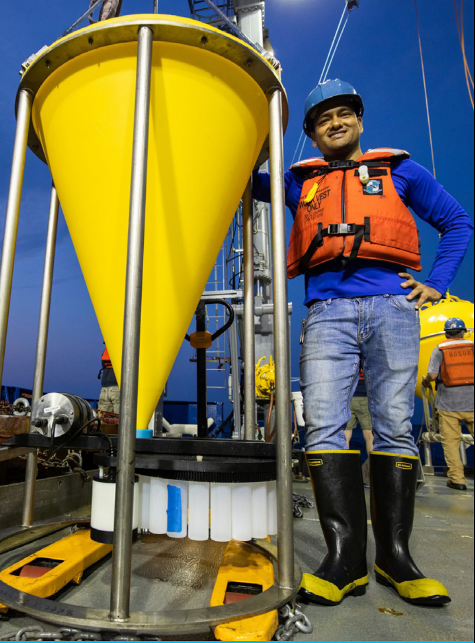
WHOI Postdoctoral scholar Wokil Bam stands tall next to a large bottom tethered trap on the stern of R/V Neil Armstrong. The trap will collect falling organic materials in the twilight zone to better understand how this layer helps the ocean sequester atmospheric carbon. (Photo by Daniel Hentz © Woods Hole Oceanographic Institution)
